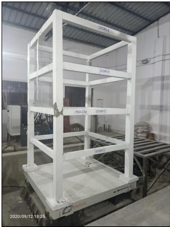
Damages after testing to 2.0g PGA
