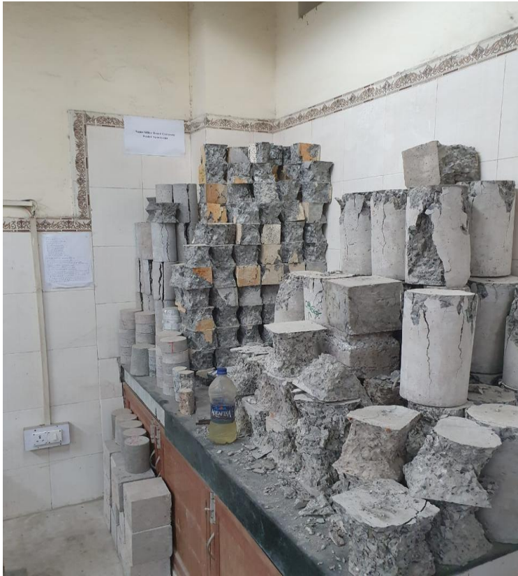
Different shape of concrete cubes after casting and testing
