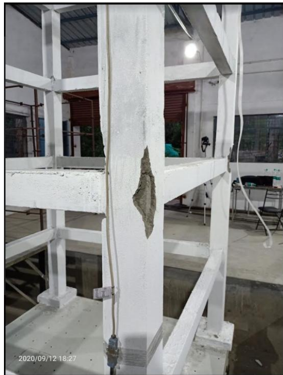
Damages after testing to 2.0g PGA
