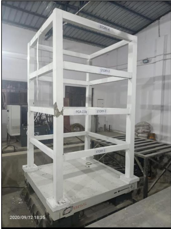
Damages after testing to 2.0g PGA
