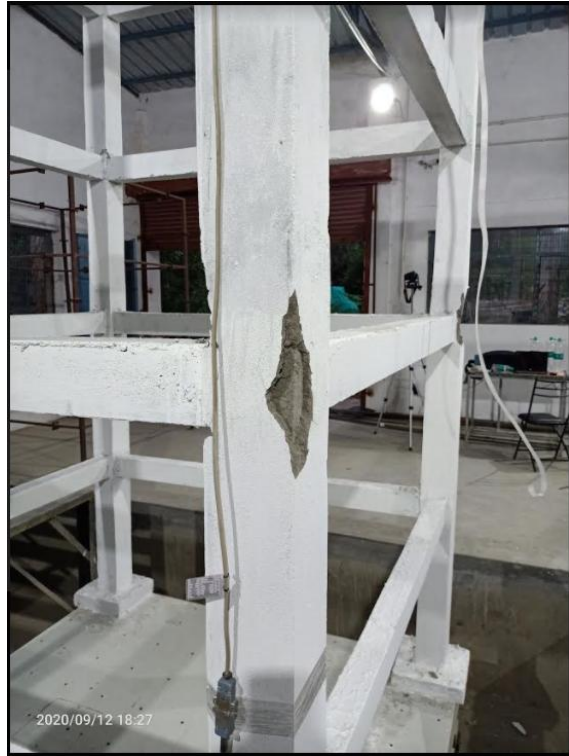
Damages after testing to 2.0g PGA
